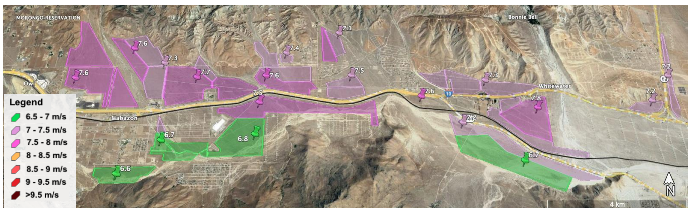
Image 3. Wind speed zones >6.5m/s (14.5mph) outside of existing wind farms at 66' (20m) above ground level
