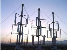
They compared the two resulting power curves, which confirmed the increased energy output from the array. Thomas named this newly discovered property the "Coupled Vortex Effect" (CVE). This discovery resulted in the awarding of International Patent US6784566 in 2004.
