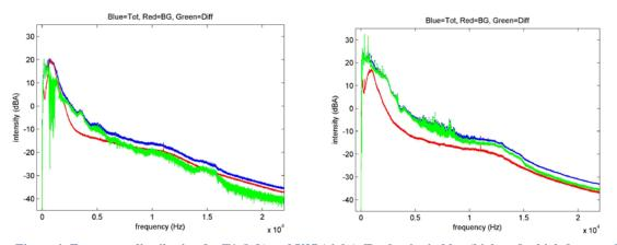
Figure 4: Frequency distribution for T1 (left) and V27 (right). Total noise in blue (highest for high frequencies), background noise in red (in middle for high frequencies) and difference between total and background noise in green (lowest for high frequencies).
