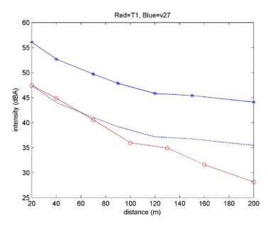
Figure 7: Noise propagation between T1 (red <sup>o</sup>) and V27 (blue \*) turbines. Dashed blue line is the blue line projected for comparison
