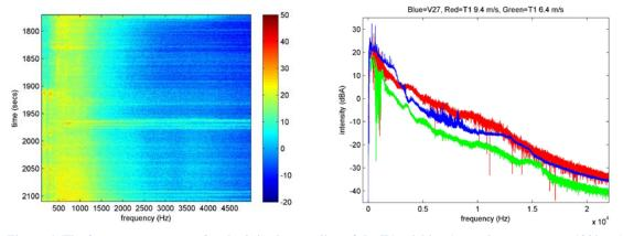
Figure 6: The frequency spectrum for the 9.4 m/s recording of the T1-tuirbine (turned on at approx. 1900 sec) and a comparison between the frequency distribution with background noise subtracted for the 6.4 m/s (green, lowest) and 9.4 m/s (red, highest for most frequencies) recordings for the T1-turbine as well as the V27 recording (blue, highest for low frequencies).
