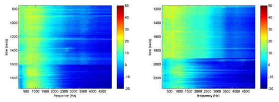
Figure 3: Frequency spectrum for T1 (left) and V27 (right). Turbines turned off at approx. 1600 respectively 1900 sec.
