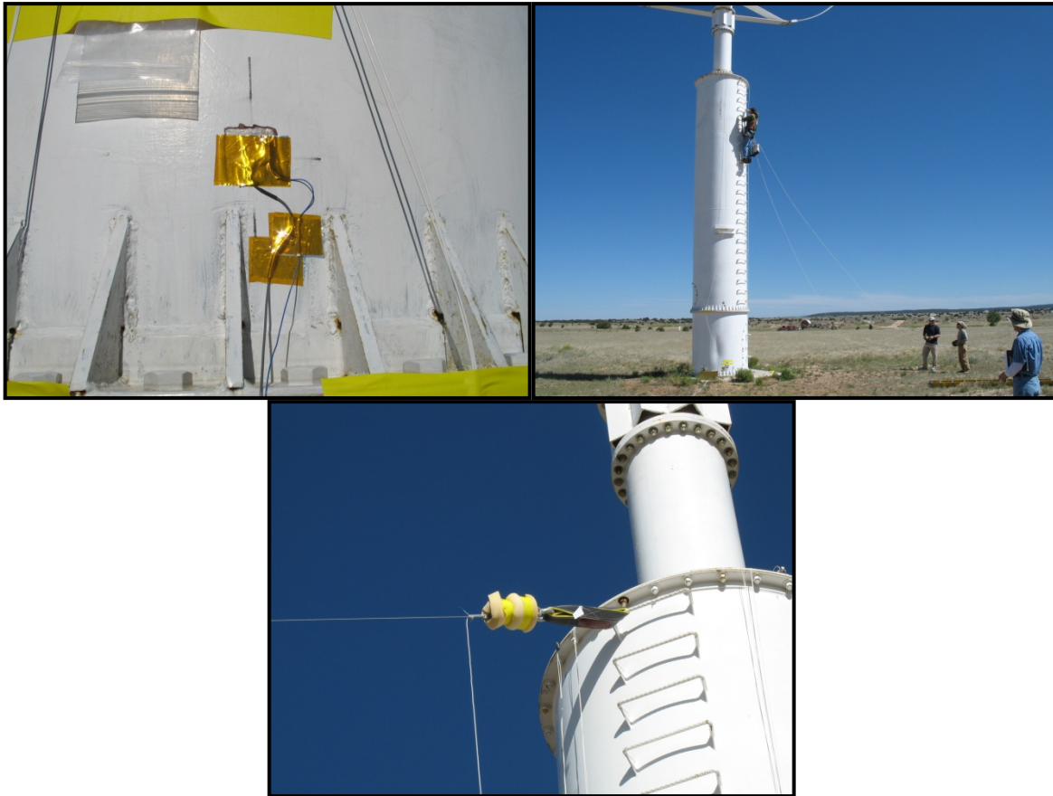
Figure 4. Photos of Instrumentation and Force Sensor a) Strain gauges at the base (top left), b) Mounting of accelerometers (top right), and c) Force Sensor (bottom, covered with foam)
