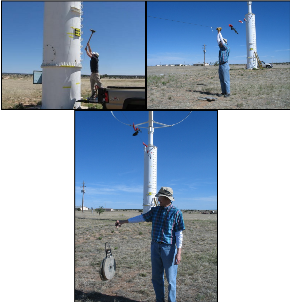
Figure 5. Photos of Artificial Excitation a) Impact Hammer Excitation (top left), b) Random Human Excitation (top right), and c) Step Relaxation (bottom)
