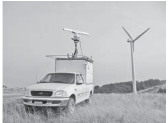
Figure 9. Mobile marine (X-band) laboratory equipped with capacity for vertical and horizontal antenna positions (B. A. Cooper, Alaska Biological Research, Inc., unpublished data). Depending upon specific applications, the antenna can be aligned in a horizontal (for assessing direction and passage rate) and vertical mode (for assessing altitude).
