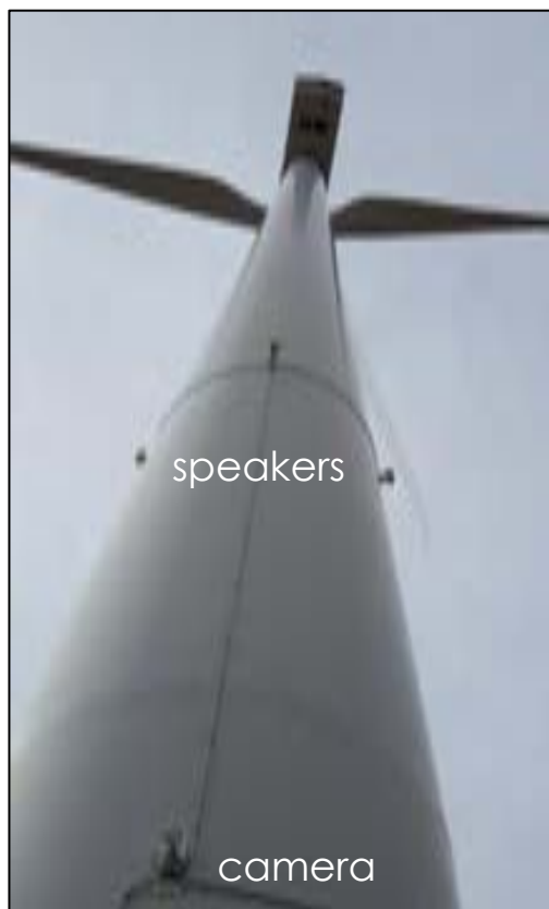
Figure 3. DTBird System Setup on a Study Turbine
